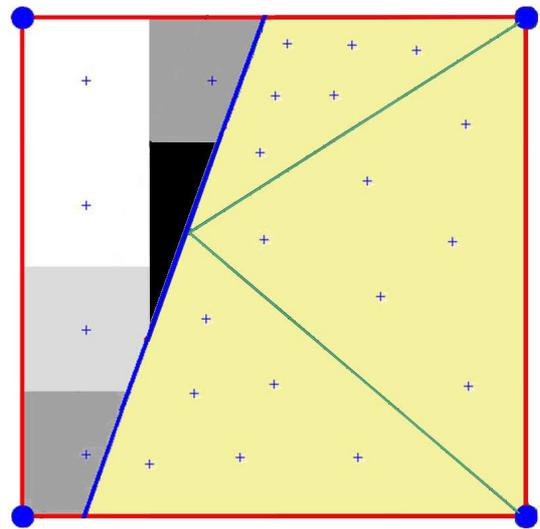
Figure 3: Integration domains and points of an element on the contour.
