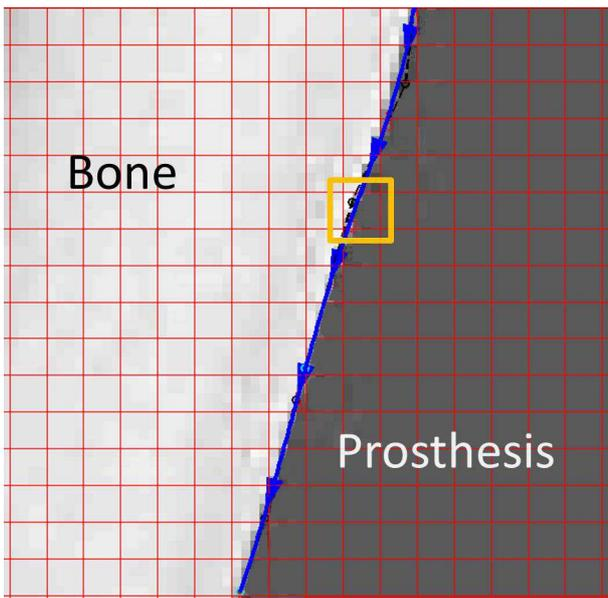
Figure 2: Homogeneous mesh of the area at the boundary between bone and prosthesis.
