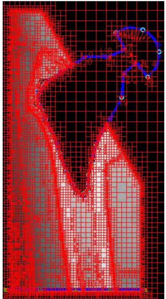
Figure 8: FE mesh of the system femur-prosthesis.
