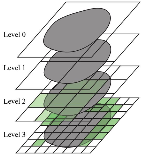
Figure 1: Hierarchical structure of Cartesian grids. Elements of different levels are used to create the analysis mesh, extracted from Nadal et al. (2013).
