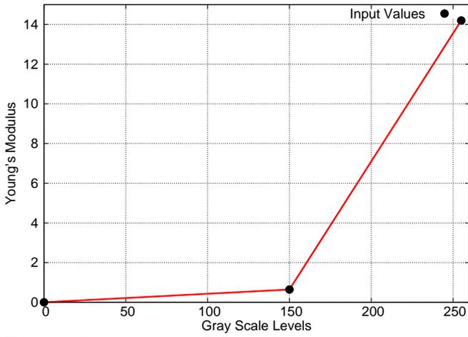
Figure 6: Interpolation of  $E$  over the gray scale.
